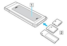
Make sure to insert a memory card into the memory card adapter in the correct direction to avoid possible damage to the memory card adapter.
